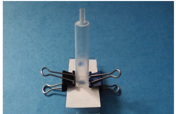
Fig. 2: A sedimentation chamber built from a slide, a perforated filter paper, a syringe and 2 strong clamps.
